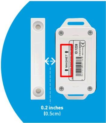
Make sure that sensor is in direct line of sight of ismartgate device. The “Status” light should be **blinking faster** when door changes position.
