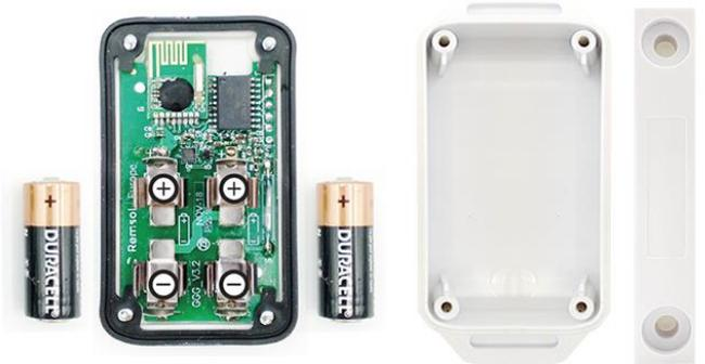
It is important to ensure that all **4 screws are tightened correctly to prevent water or moisture from entering the sensor.**
